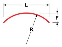
To find the value of the curved radius start from the length (**L**) and height (**F**) of the arch using the following approximate formula (**R**, **L** and **F** will be measured with the same unit of length).
